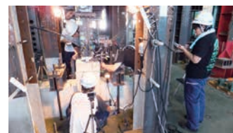
露出柱脚の基礎コンクリート周辺ひび割れに基づく損傷評価 Damage evaluation based on crack pattern and its width on the concrete foundation of exposed column base
