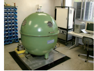
加工環境制御超精密加工機 (CAPSULE) Innovative mother machine for nano-machining
