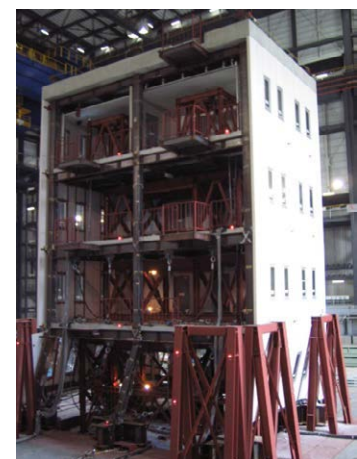
鋼構造剛接骨組の実大振動台実験 Full Scale Shaking Table Test of Steel Moment Resisting Frame
