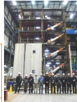
世界最大の E-Defense 震動台を用いた実物大 5 階制振ビルの実験 (神戸地震波を入力) Full-scale Test of 5-story Building with Dampers Using World's Largest Shake-table at E-Defense
