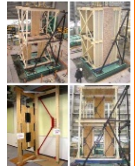
戸建て住宅制振構造の開発と実験 Development and Test for Wooden House with Passive Control System
