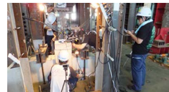
露出柱脚の基礎コンクリート周辺ひび割れに基づく損傷評価 Damage evaluation based on crack pattern and its width on the concrete foundation of exposed column base
