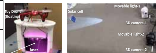
光無線給電プロトタイプ実験：(左) ドローンの浮遊中給電、(右) 複数光源システムの制御による光照射実験 Prototype experiments of OWPT: (left) Dynamic charging of drone for continuous floating, (right) Light irradiation by control of multi-light source system.
