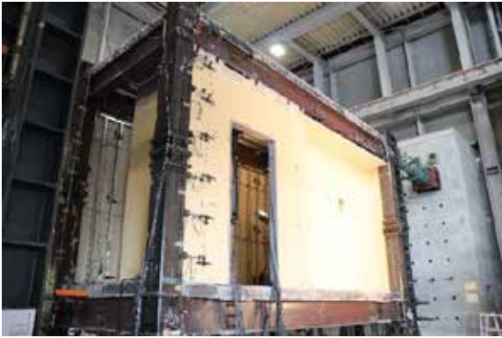
非構造部材を取り付けた鉄骨造建物の実大破壊実験 Real scale experiment of steel structure with non-structural components
