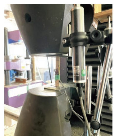
Fig. 4 Tensile Test of Bamboo at the Institute of Science, Tokyo
